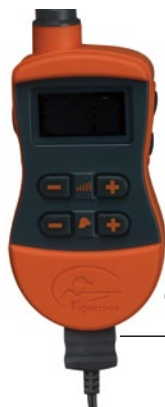
CHARGER CONNECTOR PLACED IN THE REMOTE TRANSMITTER CHARGING JACK
